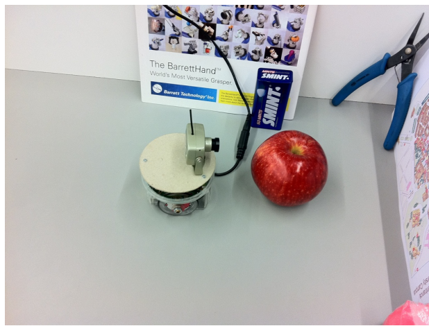
Fig. 4. One of the E-Puck's intentions is satisfied by perception of the color red. If that intention were active, this would be a rewarding state for the robot. If the other intention were active, this would not be rewarding. When the reward signal is positive, all colors detected in the image are gradually associated with the CoS for that intention. It is essential for the robot to see different background colors. Of course, if one never sees a teacup apart from its saucer, one will never understand they are two separate objects.
